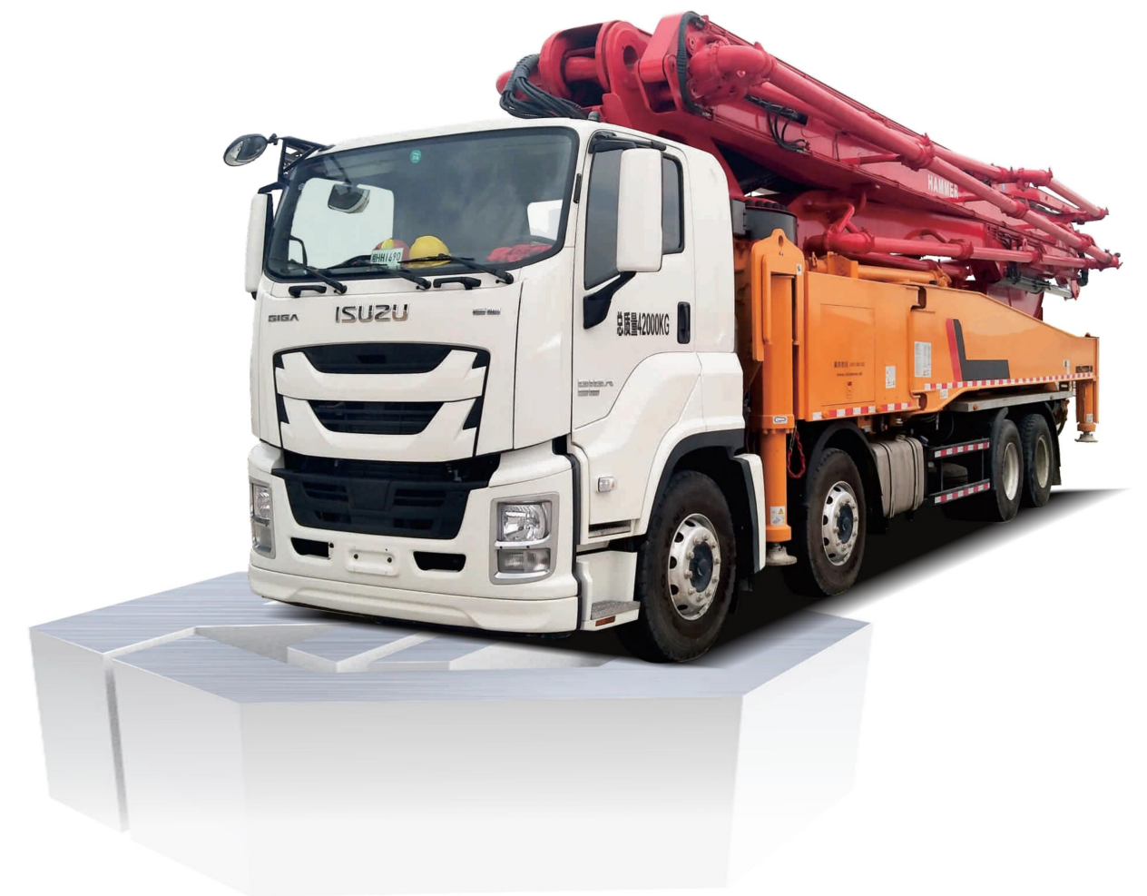
TRUCK-MOUNTED CONCRETE PUMP
