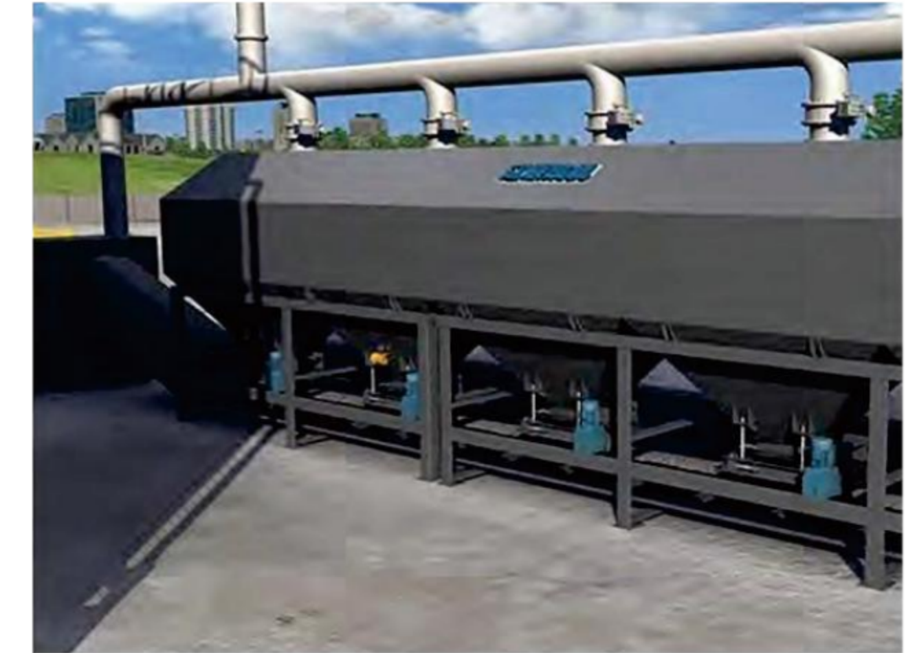
Enclosed Cold Aggregate Feeding System
