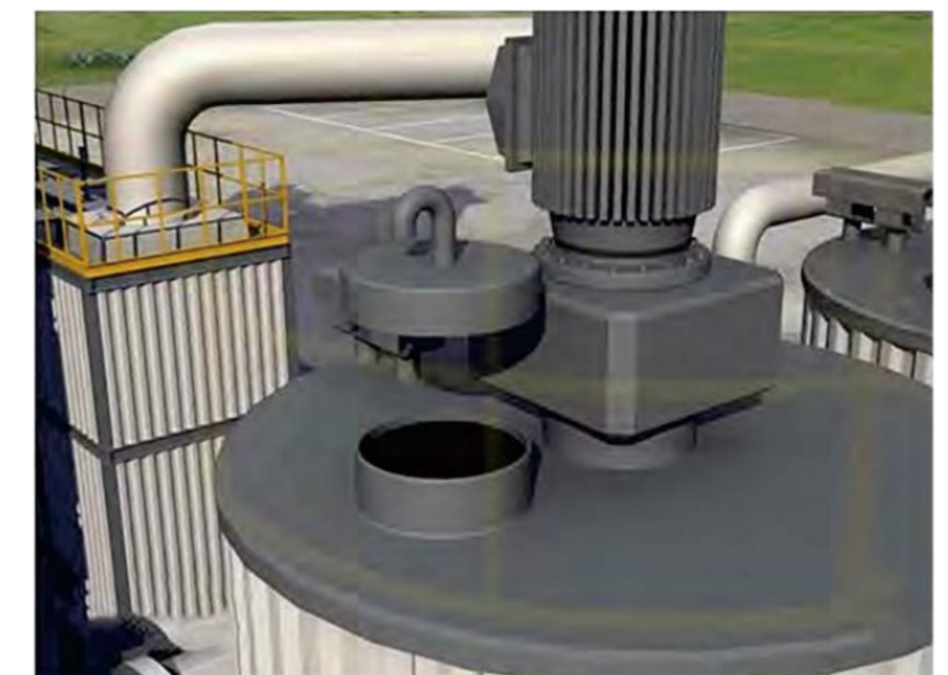
Activated carbon device, absorbing asphalt fume
